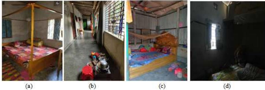
**Figure 5: (a), (b) Showing Good Daylight and Proper Ventilation Through Veranda of Brick Built Houses and (c), (d) Showing Poor Daylight and Ventilation of Low Cost Tin Walled Temporary Houses.**
